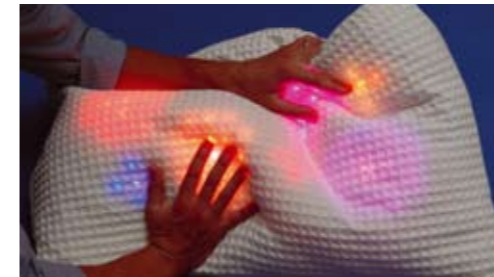
Applied in soft fabric, the light from the small pixels diffuses, resulting in more or less continuous light-emitting soft surface..
